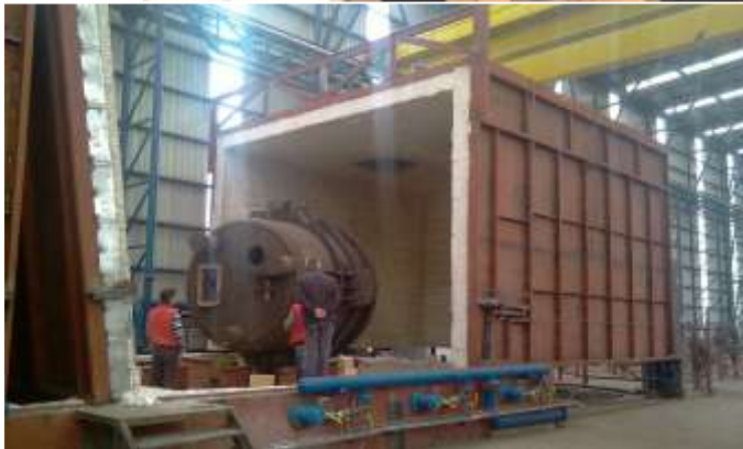
Ar Metal Post Weld Heat Treatment . Dimension: 6.500 x 15.000 x 4.500 mm
